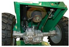
Tuff Torq™ Hydrostatic Transaxle
